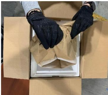
**4** Fill any low areas in the side compartments of the thermal shipping container with dry ice pellets until completely filled, so that it is equal with but does not exceed the top edges of the box that holds the vial trays.
