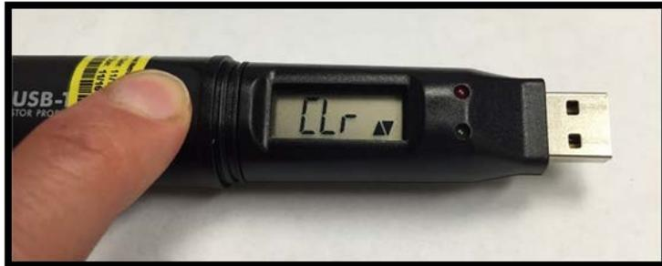
Press and hold the LCD button to clear out the previous recorded Min/Max temps. Hold until "CLr" appears on the screen. (approx 3-5 seconds).
