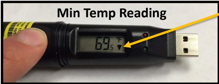
Press the LCD button again to switch the display to the Min temperature indicated by the ▼ in the bottom right hand side of the screen.
