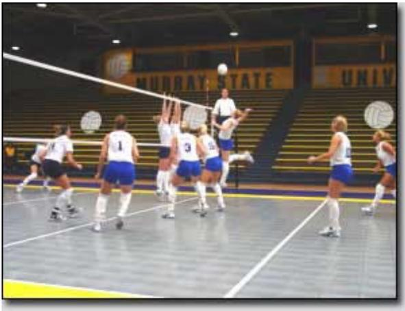
These rubber-like polymer floorings were installed in a large number of elementary and secondary schools and in colleges and universities across the country during the early 1970s to the mid 1980s. During the production of the 3M's Tartan Brand flooring, mercury was used as a catalyst to help the mixture maintain its soft texture.
